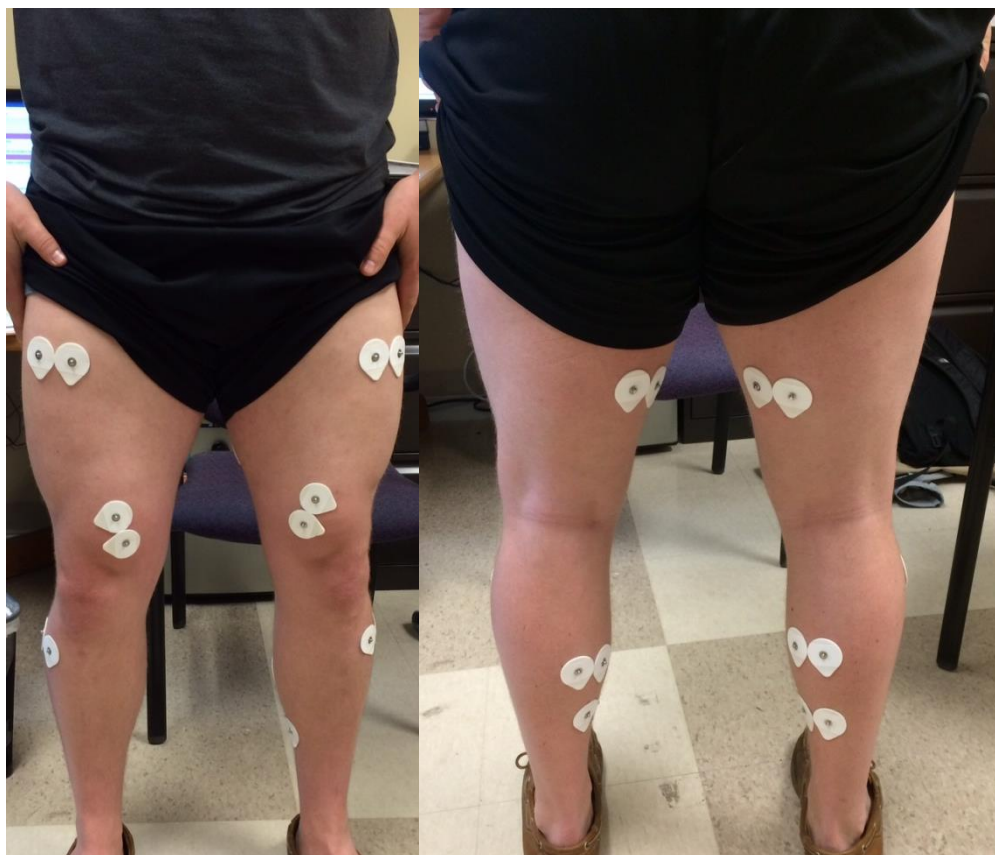
Scheme 6: Left: Anterior view. Right: Posterior view. The electrode's final location was determined on both initial muscle palpation and the visual assessment of signal quality.
